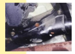
**R**emove this reinforcing shield to allow removal of the two-piece driveshaft. The evidence of ample penetrating oil in this photo betrays our aversion to broken or damaged hardware. We'd rather be oily than drill out broken studs.
