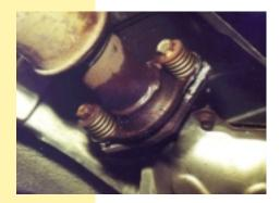
The front half of the exhaust system must be removed for clearance. Remove both spring-loaded bolts behind the catalytic converter. These special mounting nuts and bolts may be rusted together, so take your time or order a spare set of hardware for insurance before starting the job. Replace the exhaust gasket (donut) during reassembly, of course.
