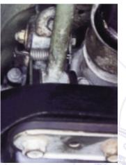
This photo reveals the Legacy's shift linkage, as well as the dummy yoke we installed at the tailshaft to keep the gear lube on the inside of the transmission. Disconnect the shift linkage, as well as torque reaction rod below it. Note the position of the shifter centering spring. You'll need to return it to this position during reinstallation of the shift linkage.
