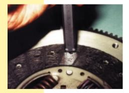
At 40,000 miles, this clutch disk still had plenty of meat left on it. The minimum allowable depth from the friction surface to the clutch rivets is 0.3 mm (0.012 inch). Also check for variations in friction material wear that would indicate a warped clutch disk. If there is evidence of oil on the clutch facings, inspect the transmission front seal, transmission case mating surface, engine rear oil seal and other points for leaks.
