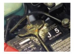
It may seem obvious, but the first step in the job is to disconnect the battery after recording the customer's radio station presets. Even a manual transmission has a surprising number of wires attached to and surrounding it. Why take the chance of damaging anything due to an accidental short circuit?
