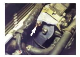
This transmission ground cable can easily escape notice. The other end of the cable is unreachable from above the transmission. A transmission case bolt must be removed to remove the ground wire at the transmission, so removing it at the body makes more sense to avoid the risk of a leak. Position the cable out of the way so it doesn't snag on anything during transmission removal.
