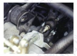
Many manual transmission Subaru vehicles are also equipped with the Hill-Holder system. This system lets the driver remove his right foot from the brake pedal after applying the brakes to stop on an incline of more than three degrees. This prevents 'rollback' when engaging the clutch to move the vehicle forward on a hill. The Hill-Holder cable shown here below the conventional clutch cable
