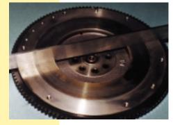
This vehicle features a flush flywheel face, although some other Subaru models have stepped flywheel designs. Resurfacing of the flywheel face to remove warped areas or heat checking is not recommended. If damage is present, replace the flywheel.
