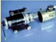
Motor and Pump Alignment
