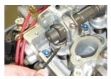
Use a micrometer to measure the thickness of the removed shim. Here's where your earlier clearance measurements come into play. To determine the required replacement shim thickness use the following formulas for intake and exhaust valve shims.
