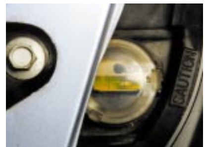
Figure 5 Vertical Movement Beam Angle Gauge
