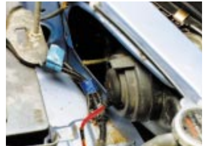
Figure 4 Vertical Aim Adjusting Screw
