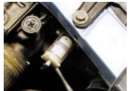
Figure 6 Horizontal Movement Beam Angle Guide
